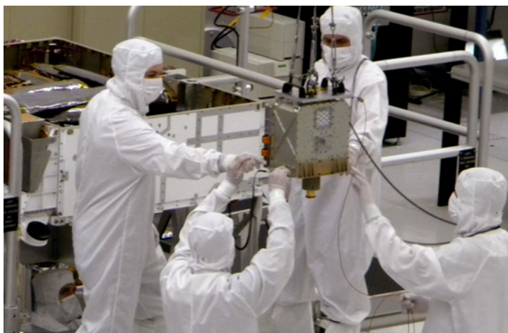
FIGURE 1 The CheMin instrument being loaded into the rover body during rover assembly. Note that for extraterrestrial use the powder diffractometer has been reduced from the size of a refrigerator to the size of a breadbox. PHOTO COURTESY OF NASA/JPL-CALTECH
